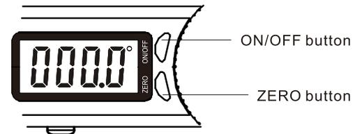
\* Automatically shut off the LCD in 5 min.
