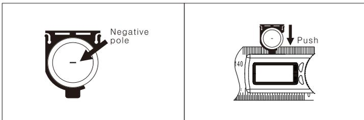
The negative pole of battery is upside, positive pole is downside.
