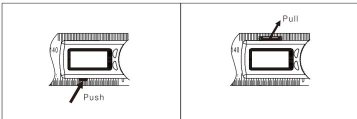
To replace battery, push the protrudent on the bottom of the LCD. The edge of battery container is shown on the upper side of the LCD
