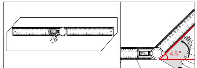
Short press ON/OFF to turn it on, put it on the flat surface as pic, make sure the both ruler's edges touch the surface, press ZERO to set zero.
